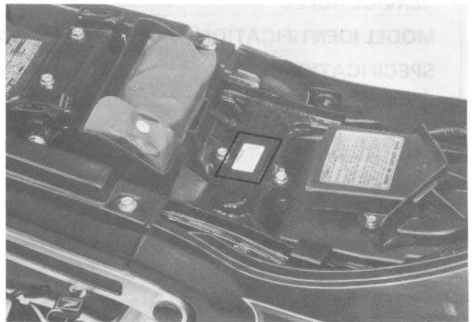
The color label is affixed to the frame under the seat.
